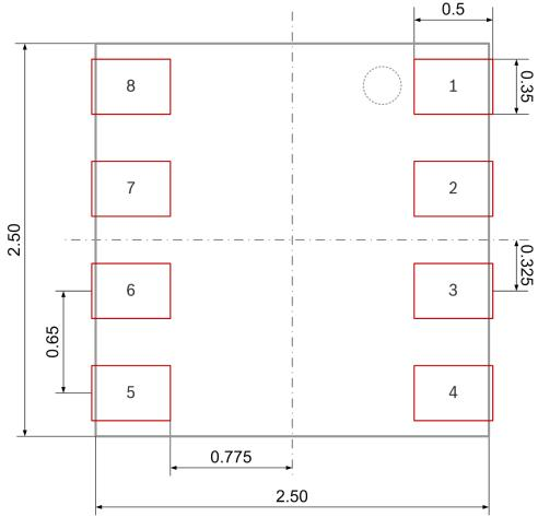
Figure 21: Recommended landing pattern (top view)
