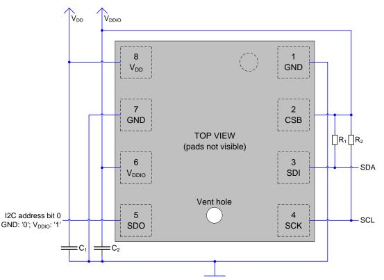
Figure 17: I<sup>2</sup>C connection diagram
