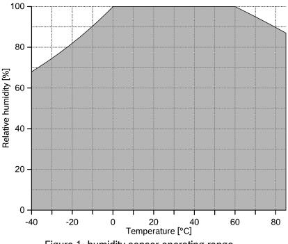
Figure 1: humidity sensor operating range
