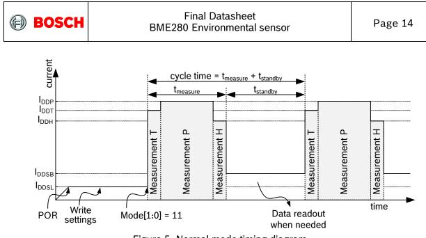
Figure 5: Normal mode timing diagram
