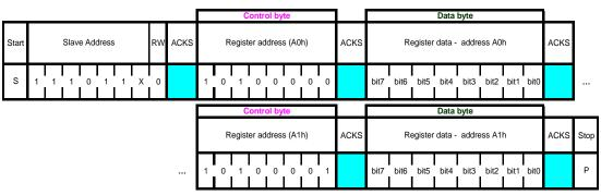
Figure 9: I<sup>2</sup>C multiple byte write (not auto-incremented)
