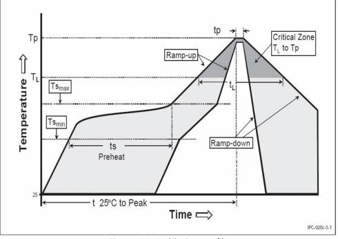
Figure 22: Soldering profile
