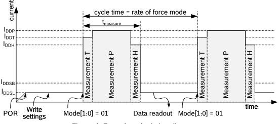
Figure 4: Forced mode timing diagram
