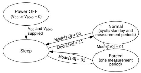
Figure 3: Sensor mode transition diagram
