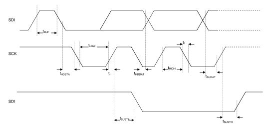
Figure 14: I<sup>2</sup>C timing diagram
