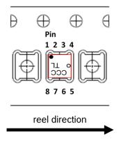
Figure 24: Orientation within tape
