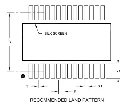
MILLIMETERS Units MIN MAX **Dimension Limits** MOM Contact Pitch 0.65 BSC Ε Contact Pad Spacing С 7.20 Contact Pad Width (X28) X1 0.45 Contact Pad Length (X28) Y1 1.75 Distance Between Pads G 0.20
