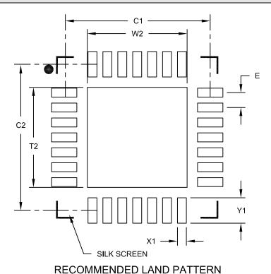
MILLIMETERS Units **Dimension Limits** MIN NOM MAX 0.50 BSC Contact Pitch Ε Optional Center Pad Width W2 3.35 Optional Center Pad Length T2 3.35 Contact Pad Spacing C1 4.90 C2 4.90 Contact Pad Spacing Contact Pad Width (X28) 0.30 X1
