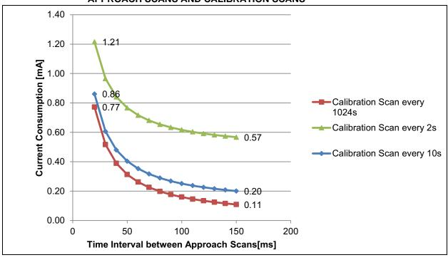
FIGURE 4-7: CURRENT CONSUMPTION FOR A FIXED TIME INTERVAL BETWEEN APPROACH SCANS OF 20 ms
