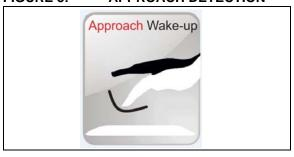
Approach Detection is an embedded power-saving feature of Microchip's Colibri Suite. It sends MGC3X30 to Sleep mode and scans periodically the sensing area to detect the presence of a human hand.
