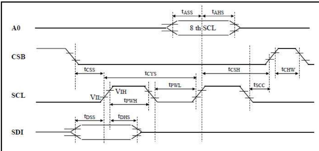
NOTE : The input signal rise time and fall time (tr, tf) is specified at 15 ns or less.
