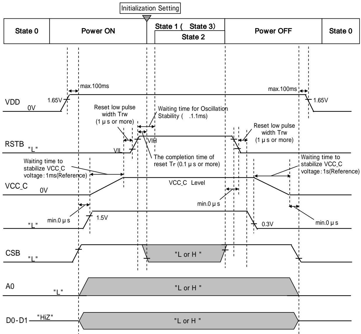
NOTES: - If VDD is turned on but nothing is displayed, the OLED unit shall be put into State 1 or State 3.
