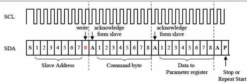
Figure 5. Write Single Parameter Command
