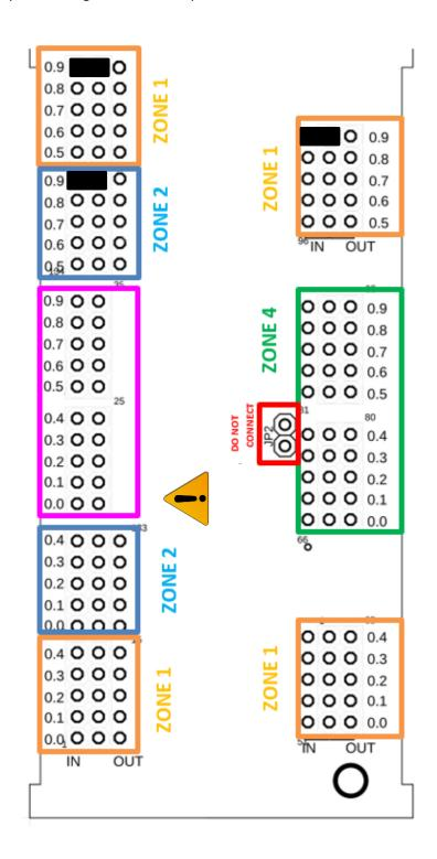
This is an exemple to configure 0.9 as an output.
