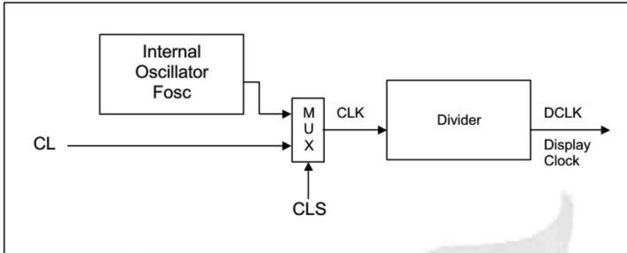
Figure 9 - Oscillator Circuit
