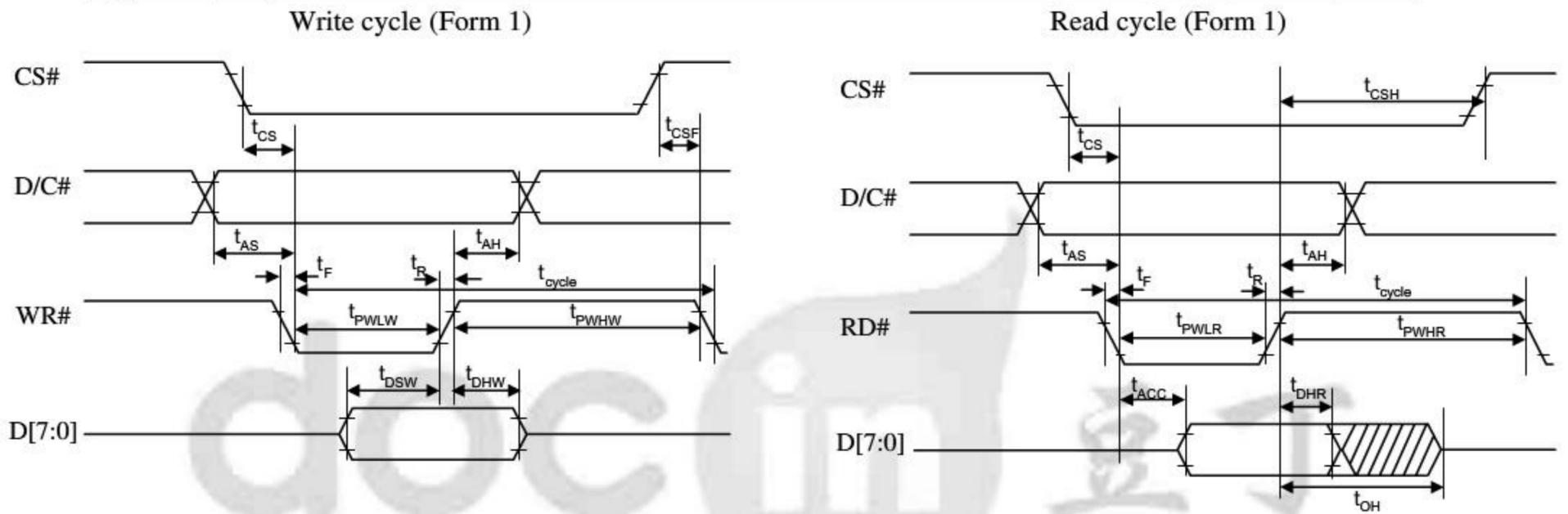
**Figure 38 - 8080-series parallel interface characteristics (Form 1)**
