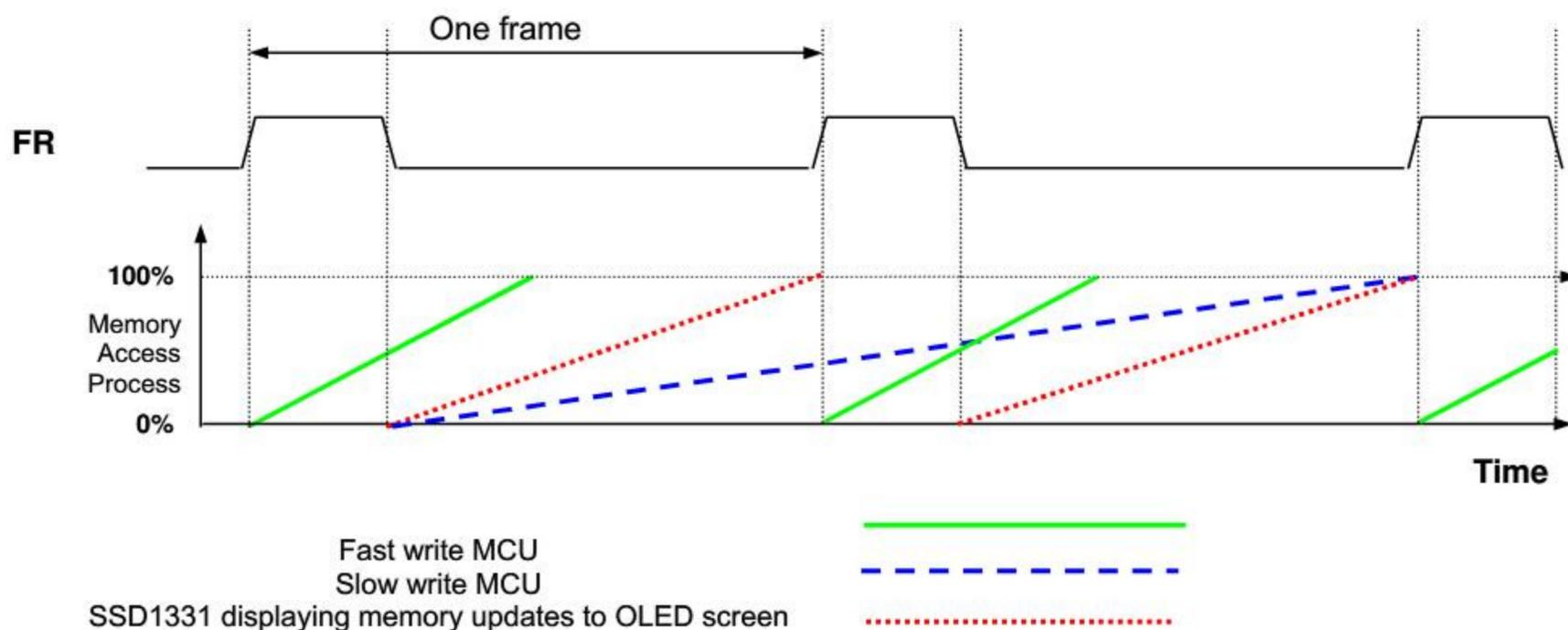
The starting time to write a new image to OLED driver is depended on the MCU writing speed. If MCU can finish writing a frame image within one frame period, it is classified as fast write MCU. For MCU needs longer writing time to complete (more than one frame but within two frames), it is a slow write one.
