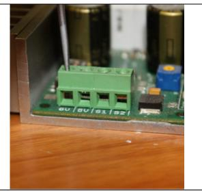
**Step 1:** Strip the wire which you are using approximately <sup>1</sup>/<sub>4</sub>" The wires may be 14 gauge to 30 gauge
