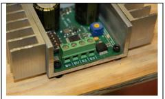
Figure 2.3: Mounted to a wood frame using standoffs
