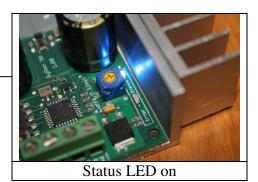
selected, the status LED blinks the number of cells detected. Unless you are in lithium mode, the status LED will usually remain on.
