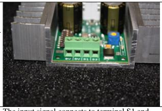
The input signal connects to terminal S1 and sometimes S2
