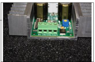
The 5V terminal can be used to power small loads, like a potentiometer or a radio receiver. The 0V signal must be connected to the ground of the device generating the input signal.
