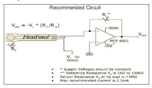
In the circuit shown, the dynamic force range of the sensor can be adjusted by changing the reference resistor  $(R_F)$  or by changing the Drive Voltage  $(V_O)$ . Refer to the Saturation section for additional information.
